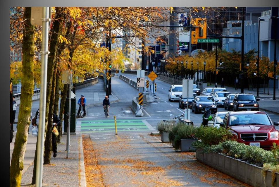
Note the bike parking integrated with the cycle track curb, which doubles as a pedestrian bulb-out. Very clever.
